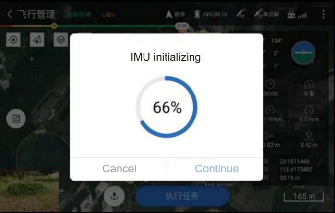
c. LiDAR self-check and IMU initializing on GCS(no need 8-shape check).
