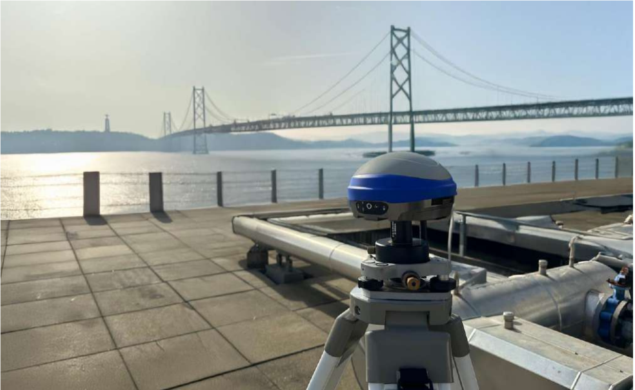
Figure 12 - Viking installed on a tribrach.
