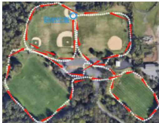
Schematic Diagram of Block-Wise Scanning for Large Outdoor Scenes
