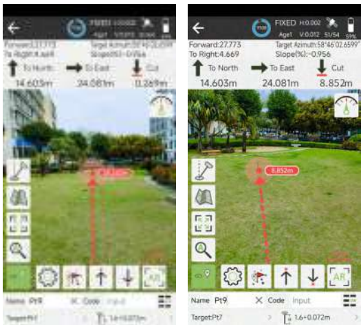
Remote AR-Guided Staking-out
