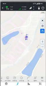
Select points to form a polygon, and directly identify the area division points for the surveyor to stake out. There is no more need for the user to guess a position to measure, and then to adjust.
