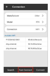
"Fast connect" means handheld controller could find your nearest GNSS receiver and connect fast by NFC. You do not need to choose any of receivers on screen.
