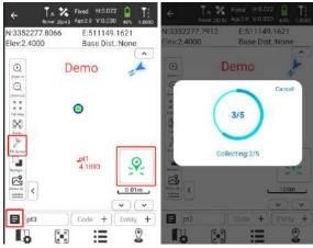
In addition, Tilt Survey is also supported. After initializing IMU you could tap to capture your point. Tapping you could find "Points" which you have been collected.
