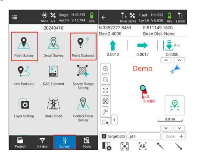
In Point Stakeout, you could see the direction clearly which you need to go forward or backward or ground filling.
