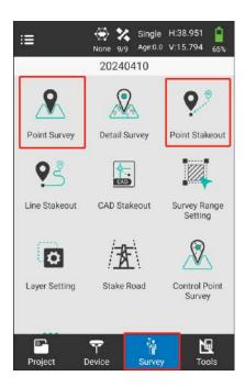
Currently, we have three surveys and three stakeouts. You could choose any of them to survey in your work according to your requirements. Now I take Point Survey and Point Stakeout for an example.
