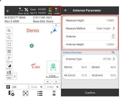
At first, it is necessary to set the height of antenna. Tap 1.8000 and change antenna parameters. the whole figure of measuring methods is as follow.
