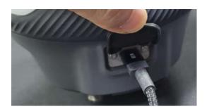
If the device is powered on and connected to a terminal device such as a computer via a USB cable, you can access the memory drive within the device through the file manager for file management.
