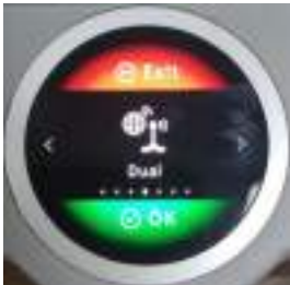
Dual transmit (inbuilt radio and cellular network)
