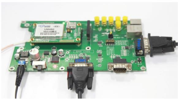
Figure 4-3 Connect the Serial Port
