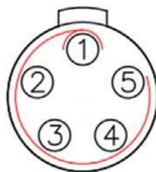
Figure 7 HJ394 C Port Welding Surface View
