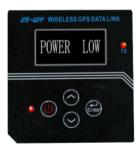
Sleep mode: If there is no any operation on the radio buttons for 10 minutes, the display will shut down to save power, the power indicator is still on, and TX indicator is still continue blinking.
