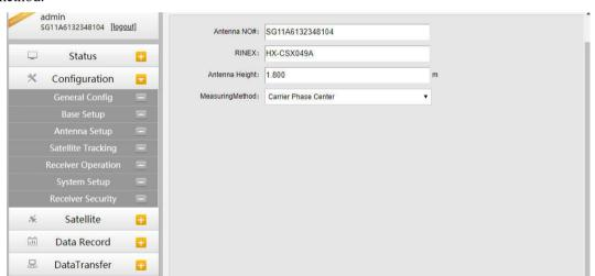
Antenna Height: This is the value for height of antenna while surveying.
