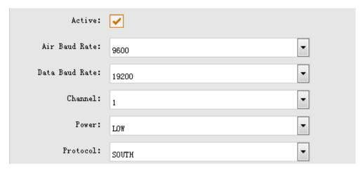
3, configure the datalink of the other rovers into internal UHF mode, then make sure the channel, protocol and frequency point are same as "Route" rover.
