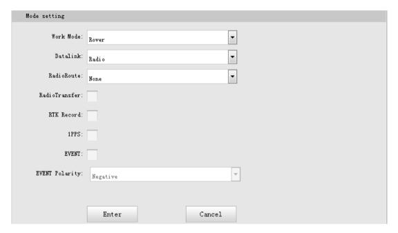
Work Mode: There are Rover, Base and Static contained in this dropdown list
