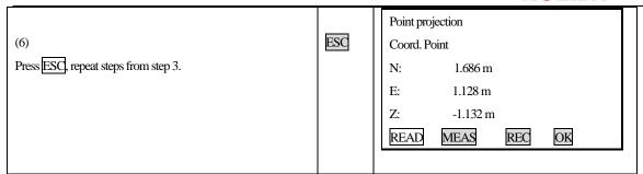
**Note:** It is possible that you don't have known point coordinates to set station and backsight point. You can assume a Station Point coordinate, input angle to set backsight point. Then measure the start point and end point to get their coordinates, use them when you are designing baseline.
