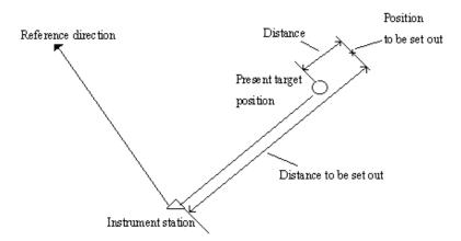
·From the menu mode, selecting "2. S-O" also can perform setting-out measurement.
