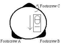
3 Repeat the procedures 12 for each 90°(100g) rotation of the instrument and check whether the bubble is correctly centered in all directions.
