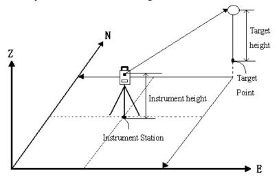
It is possible to set the azimuth angle of a backsight station by entering the coordinates of the instrument station and a known point (backsight station) and then sighting at the backsight station.
