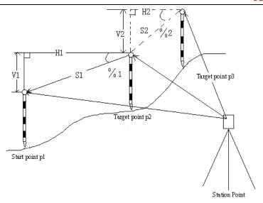
·To find the height difference between 2 points, use a pole to make the target height of all the targets identical.
