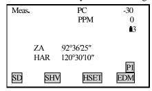
When the preparations for measurement are completed, the instrument is in MEAS mode.
