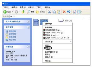
(5)Enter removable disk H, paste the file to removable disk by selecting the copied item in the popup menu. Moveover, the popup menu also supports the deleting and editing of file data. By pessing [ESC] on the keyboard of KTS-442UT, disconnects the computer and returns to data communication menu.
