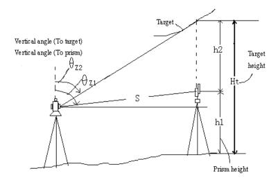
·The height of the target is calculated using the following formula.
