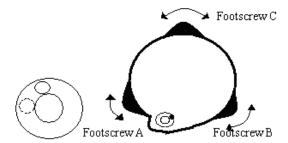
①Turn the leveling screw A and B to move the bubble in the circular level, in which case the bubble is located on a line perpendicular to a line running through the centers of the two leveling screw being adjusted.
