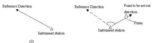
Operating Procedure Operation Display Meas. PC -30 PPM (1) Sight the reference direction, press Oset twice **1**3 in the second page of MEAS Mode. The 0set ZA 89°59′54" horizontal angle of the sighting direction is 0. HAR 0°00′00″ 0set SD **OSET** SHV S-O Observation (2) Press S-O in the second page of "MEAS 2. Set-out 3. Stn data Mode Screen". The "Setting-Out Measurement S-O Set h angle Menu Screen" is displayed. EDM
