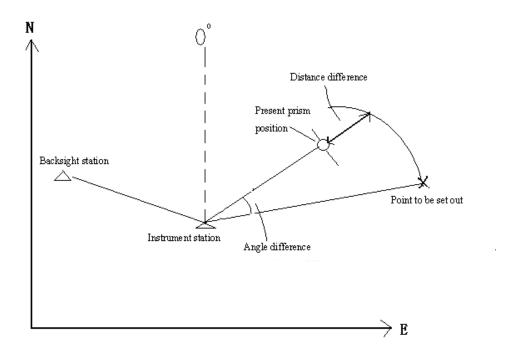
It is possible to perform coordinates setting out measurement by selecting "2. S-O" from Menu Mode. It is possible to output the coordinate data previously entered and set it as the setting out coordinate. To find the Z coordinate, attach the prism to a pole, etc., with the same target height.
