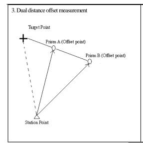
·Install the offset point A and B on a line extending from the target point, measure A and B, then enter the distance between B and the target point to find the target point.
