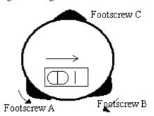
② Rotate the instrument 90 (100g) around its vertical axis and turn the remaining leveling screw or leveling C to center the bubble once more.
