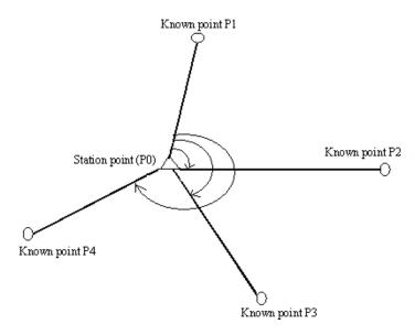
The KTS-442UT can calculate the instrument station coordinates by observing 2 to 4 known points.
