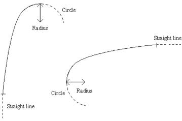
Press TRNS key in the "Main Line Input Screen", the transition curve can be defined. Transition curve consists of the minimum radius and arc length. The rule of radius value: along the forward direction of the curve. When the curve rotates to right, the radius value is positive. When the curve rotates to left, the radius value is minus. The arc length can not be minus.
