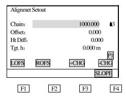
**SLOPE:** The key is used in slope set out. (Press FNO key)
