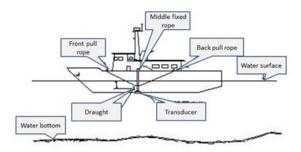
The position of the fixed transducer is best selected next to the middle side of the hull, avoiding the noise interference of the hull as far as possible, and then fixing it by pulling the rope at the front, rear and bottom.
