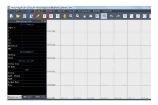
If there is no information come, please check the configuration in "setting – survey devices" again, and check the EchoSounder and Hysurvey software is not expired in "Register".
