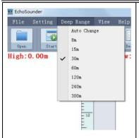
Depth range is important for auto survey mode, and you need to select the correct range to let KOLIDA echo sounder adjust the sounding parameters automatically.
