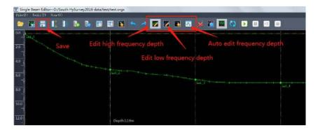
After you open the line file, you can click the "Auto" process first, then you can check by manual. If you find some echo wave error, use the edit high or low depth to edit it back to normal. After finishing edit 1 line, click "Save" to save the data, and open another line to process.
