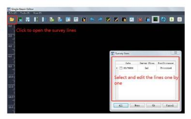
Opened the line file and check the data, if find some false data, you can use the edit tool bar to edit the data.
