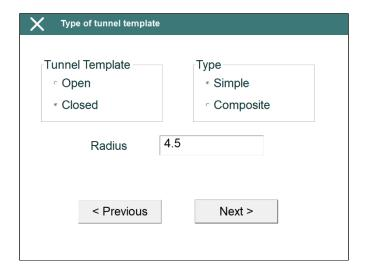
Only the *Radius* value should be entered for simple cross-sections, while *Radius* and *Sidewall* length should be entered for composite cross-sections. In the latter case, the cross-section will be created with straight sidewalls that start at the left-hand and right-hand points of the semi-circle having the radius indicated.
