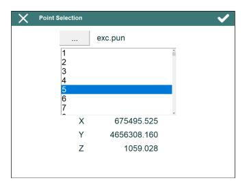
*Manual*: Allows one to manually enter the coordinates of the point to be set out. This point can be saved in the current file by clicking on the record button. It will be assigned with the number of the last point plus 1.
