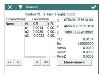
The user must enter the accuracy parameters of the total station before make the calculation. This option is available within the menu of the title bar, y allows one to set up the values for calculating the uncertainties of the angle and distance measurements.
