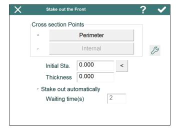
The user can select points on the tunnel template (*Perimeter*), or inside it (*Internal*). In the first case, there are several methods (see Features and Functionality > Theoretical Points of the Tunnel Template).
