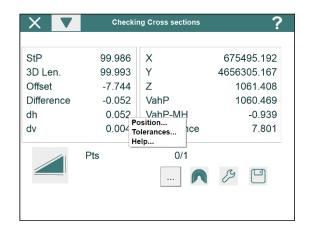
When click on information button and select a measured point, the program shows the station and the coordinates X, Y, Z of that point and, also, the total station rotates to that point.
