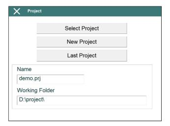
**Last Project:** This option selects the project worked in the last session. In this case, the application shows the *Name* and the *Working Folder*. When the application is initiated for the first time or when the program's initial configuration is restored, it appears as deactivated.
