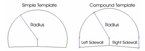
Of these, only the first two can be defined in the field data recorder itself. Complex cross-sections have to be created with the TcpTunnel CAD program. All cross-sections created in this module will be treated by the application as if they were complex, even if they are simple or composite cross-sections.
