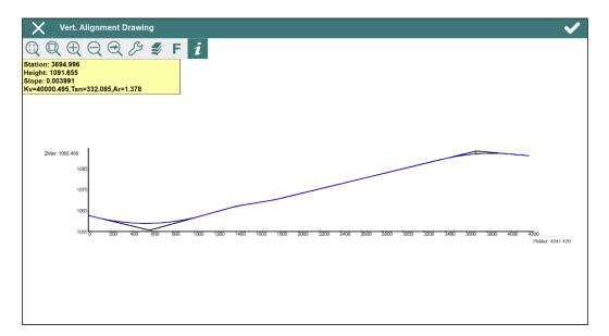
The button with the letter **F** allows different scale values for the drawing.
