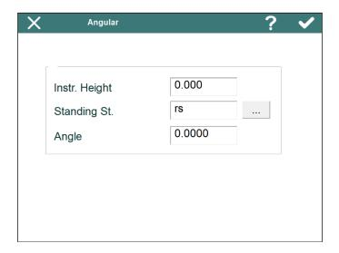
Should it not be possible to set the azimuth indicated at the station, information will be provided about the horizontal correction that will be applied to each observation.
