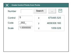
The number of the desired point should be entered in the **Number** box and the *Search* button or the button should be clicked and the point selected from the list shown. The button adds the control point to the selected file.
