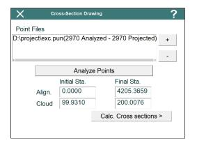
At first, the user must select the files which stored the points to be analyzed. The buttons allows user to add and remove, respectively, files from the list. Then, the *Analyze Points* button must be pressed. After finishing this process, the program will show the initial and final station which is the point cloud. The next screen of the wizard will be showing by clicking on *Calc. Cross Sections* button.
