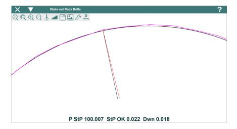
For each measurement, the program draws, in black color, the theoretical position, and, in red color, the measured one.
