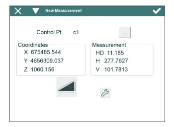
Also, with motorized total stations, the program allows to rotate automatically the total station for doing the reverse measurement and for looking for the selected control point after 2 or more control points have been measuring.
