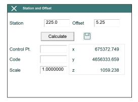
The coordinates of a new control point are shown on screen by entering a *Station*(chainage) and *Offset* and clicking on the *Calculate* button. A name should be entered for the control point and the button clicked to save the data.
