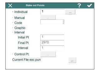
The name of the project's current points file is shown in the lower part of the screen. Clicking on the \_\_\_ button allows one to select any other points file.
