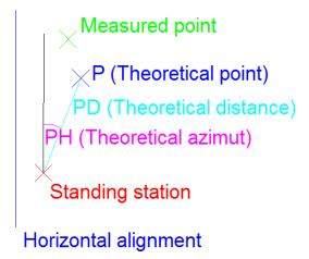
The staking out is performed in the same way as in the setting out **Points** option, appearing in this same chapter.
