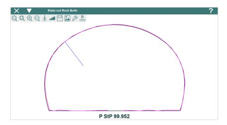
The following measurements must be done pointing to a guide. The objective is to position this guide online with the calculated station and perpendicular to tunnel template. For doing this, the program shows the movements to do forward (Fwd) and backward (Bwd), to reach the station (StPOK), and up (Up) and down (Dwn), to reach the position of the bolt.
