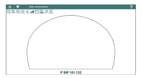
For each theoretical station, the program shows the tunnel template that has been assigned to that station and the measured profile if the point file contains points within the tolerance. The first drawing is the tunnel template assigned to the initial station of the horizontal alignment.
