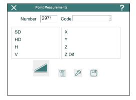
The *Number* of the point (alphanumeric) must be entered and, optionally, the *Code*, which can be selected from the program's database.
