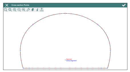
On the other hand, the program allows one to define theoretical points by entering a horizontal and vertical offsets regard to horizontal and vertical alignment application points. These points can be entered manually or import them from file. Each line in the file must have the format: **number h\_offset v\_offset**. A blank space must be entered between fields.
