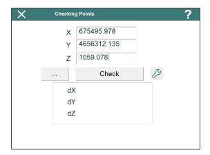
To start this process, one must set a point coordinates, by clicking on button, and click the *Check* button. One is first asked to check the position to ensure the correct point is aimed at and then an measured is performed from the station to check the point.
