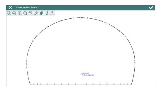
The blue points indicate the cross-section's unique points, and the red points indicate the points calculated from the keystone on the basis of the increment indicated.
