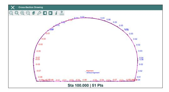
Before starting survey, several setting parameters can be modified through the option included in the menu of the title bar. Apart from the mentioned parameters, station tolerance and number of iterations, messages related measurement errors and points out of tolerance can be disabled.
