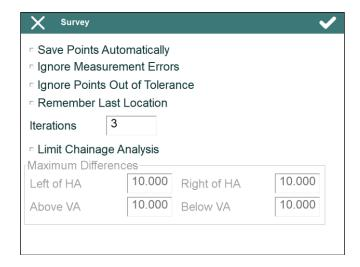
**Save Points Automatically**: Each measured point within **Survey > Point** and **Checking > Cross sections** options will be stored automatically after measuring it, otherwise, several measurements can be done without stored the point.
