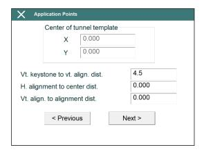
Vertical keystone to vertical alignment distance: A positive value should be indicated if the keystone point is above the vertical alignment and superelevation application point and negative otherwise. Under normal conditions, this value should always be positive. The vertical alignment and superelevation application point should be within the tunnel template.
