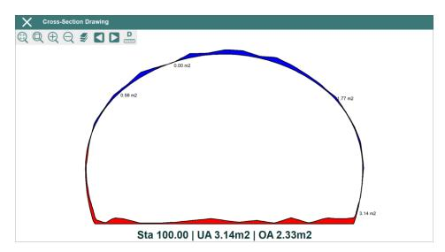
The program shows the *Station* and the number of points for each cross-section if *Calculate Areas* option is not checked. Otherwise, the program shows information about underbreak (UA) and overbreak (OA) areas.
