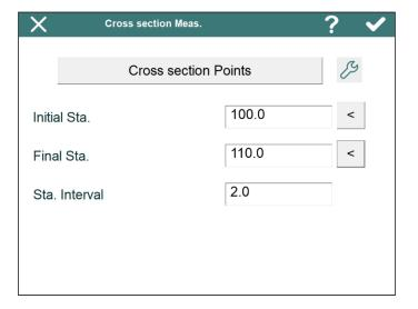
*Initial Station*: The station can be measured by clicking the station.
