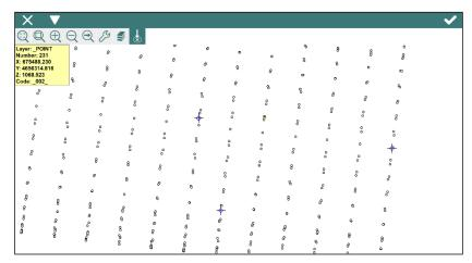
*Interval*: Allows one to set out from the initial to the final point in accordance with the interval entered. This marks the number of positions jumped within the file.
