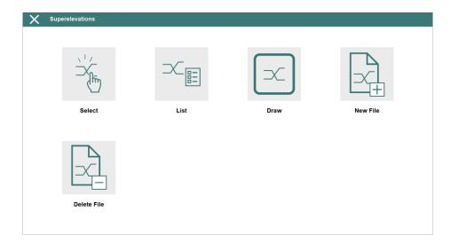
These files contains the superelevations of the project to rotate the tunnel template or to apply to the height when staking out roadbed. They have \*.PER extension and are compatible with **TcpMDT** and **TcpTunnel CAD** files.
