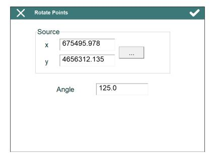
**Source:** The base points coordinates should be entered either manually or by clicking on the button.
