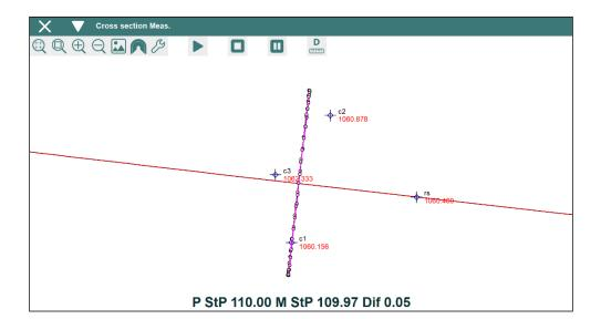
After survey finalized, a graphic with theoretical and measured cross sections is shown.
