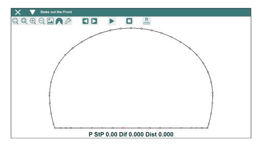
**P** StP: Theoretical station of the cross section (or profile).
