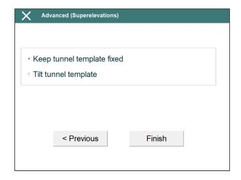
*Keep tunnel template fixed*: The tunnel template doesn't rotate with superelevations.
