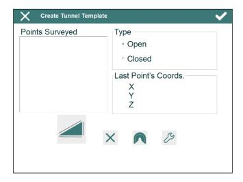
The *X*, *Y* and *Z* coordinates are shown for each point observed.
