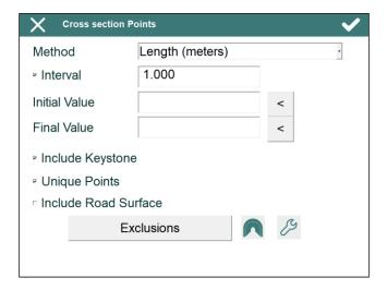
**Method**: Shows the three methods indicated above: **Angle (degrees), Height** (**meters**) and **Length (meters)**. In the case of angles, gons or decimal degrees will be displayed, depending on the option selected in **Settings** > **Units of Measurement**.
