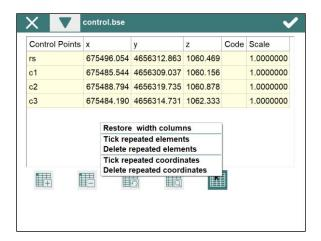
These options allow user to restore the default width of columns and locate and remove points that have the same number or coordinates.
