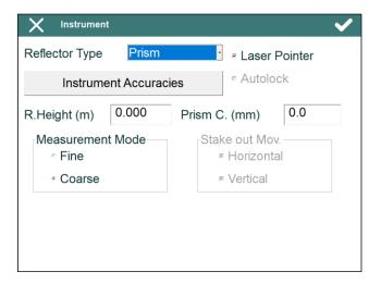
**Reflector Type:** Depending on the total station features, the program will show **Prism**, **Reflector Sheet**, **Reflectorless**, etc.
