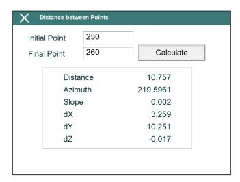
By entering two numbers and clicking on the *Calculate* button, the following information is shown on screen:
