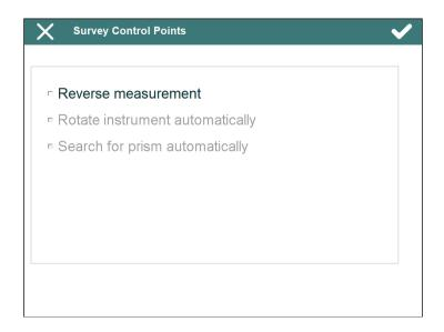
After doing a control point measurement, this one is added to **Calculation** list. The parameters will be calculated automatically if 2 or more control points have been measured.
