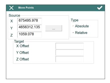
Source: X, Y, Z coordinates of the base point. The button allows one to select the point in different ways.
