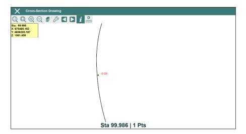
**Position** function, in the title bar menu, allows to rotate the total station to a theoretical point of the cross section on a entered station for checking this point.
