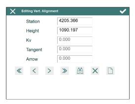
The Kv or Radius, the tangent and the arrow are automatically calculated in manual entry when one of them is entered. Depending on the type of vertical alignment file's transition curve, the Kv (parabolic transition curve) or Radius (circular transition curve) is shown on screen.
