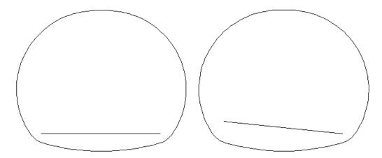
*Tilt tunnel template*: Taking the pivot point to be the point where the vertical alignment and superelevations are applied, the cross-section will tilt according to the superelevation of the station in question. This superelevation is calculated by averaging the superelevations on the left and right.
