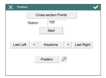
To define the theoretical points into which the tunnel template is divided, the user must enter the theoretical station and click on *Cross-Section Points* button (see **Features and Functionality** > <u>Theoretical Points of the Tunnel Template</u>).
