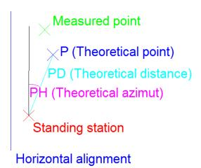
If the point is not in line, the program displays a prompt with the angle that the station must be moved to the right or to the left. In motorized stations, this information is not shown if the *Horizontal* and *Vertical* options have been selected in the <u>Instrument</u> section. The station will automatically move to the theoretical point.
