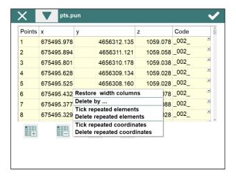
The **Delete by...** option shows a new dialog where the user can select the items to be deleted. The selection can be made indicating a range of numbers (**Select by Numbers**) or by entering a code (**Select by Code**)
