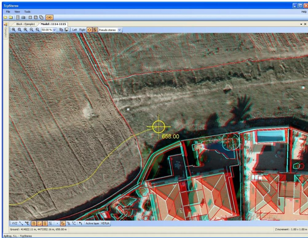
Figure 36 – Plotting 2D contours.
