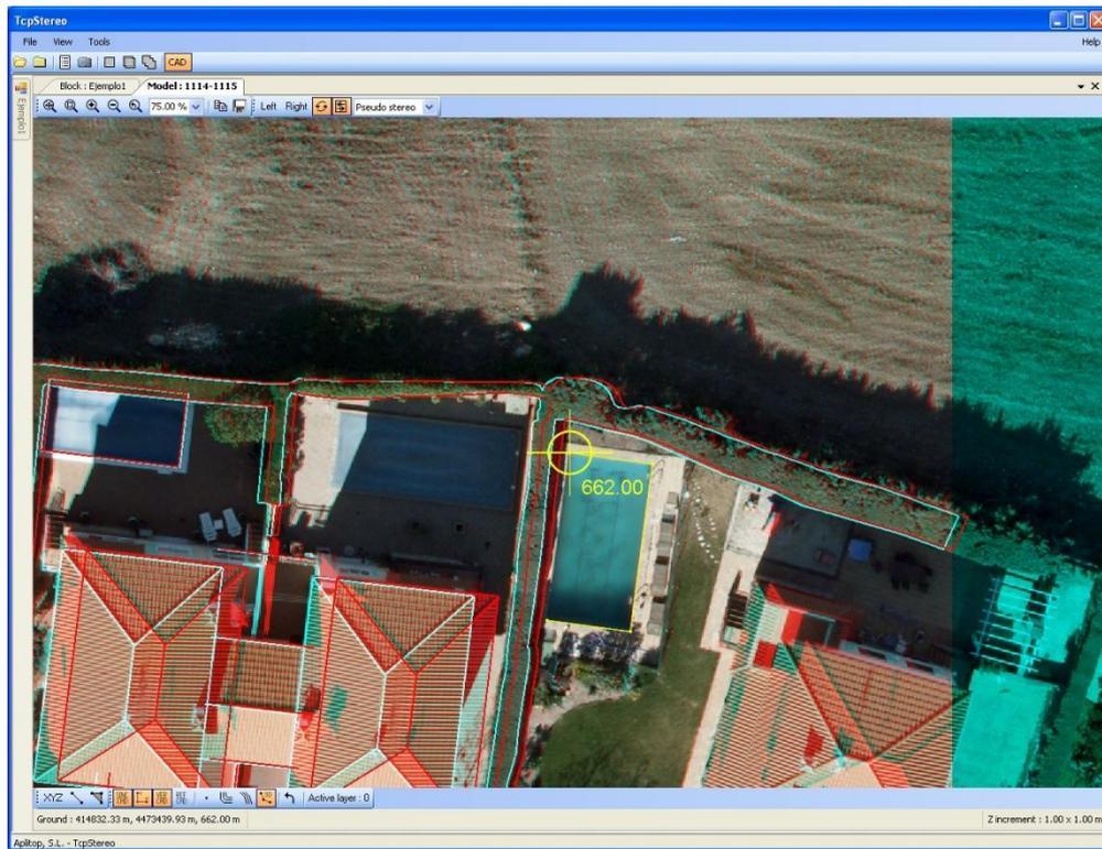
**Figure 38 – Plotting 3D lines.**
