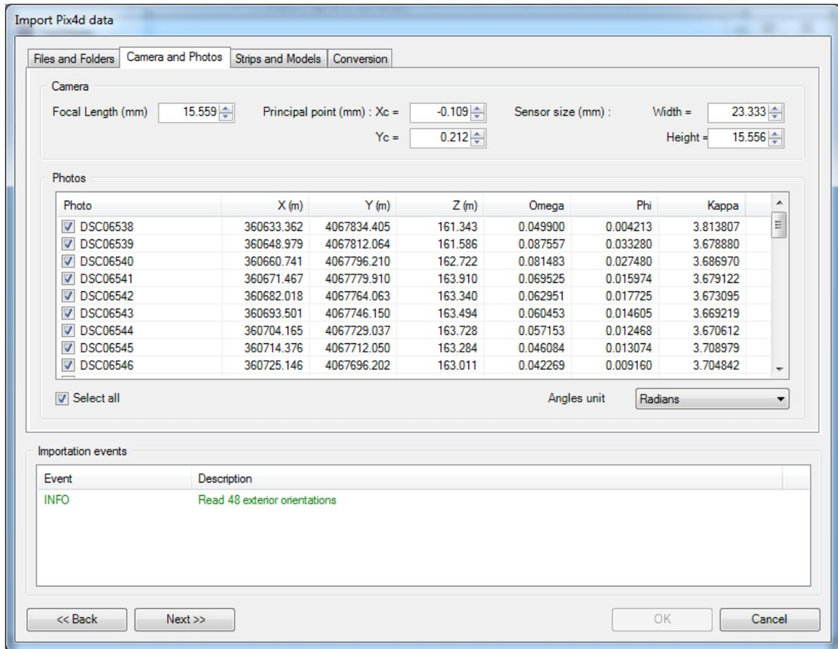
Figure 16 – Import Pix4d data: Camera and Photos
