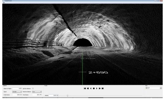
By means of a panel it is possible to control the position over the horizontal alignment being able to advance, move back, stop, go to the first or to the last station, or enter it directly.
